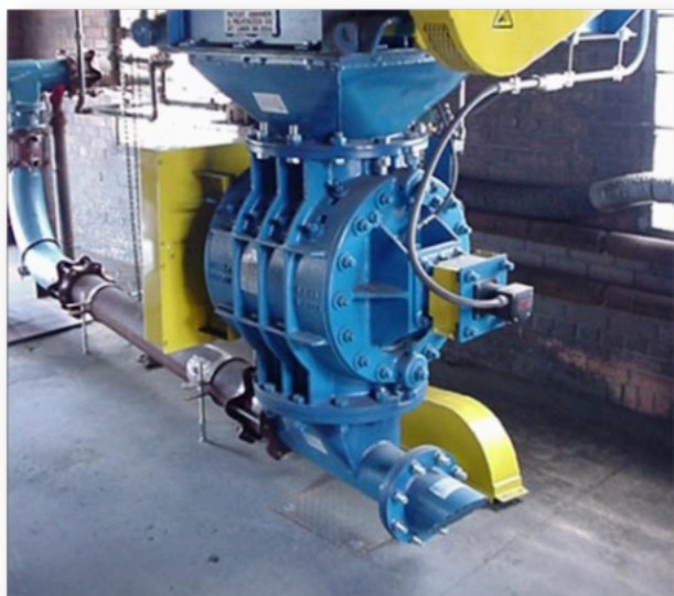
Rotary Valve Feeding a Vacuum Pneumatic Conveying Line
