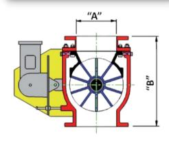
Other Manufacturers 8" Rotor vs. Type "HD" Rotor
