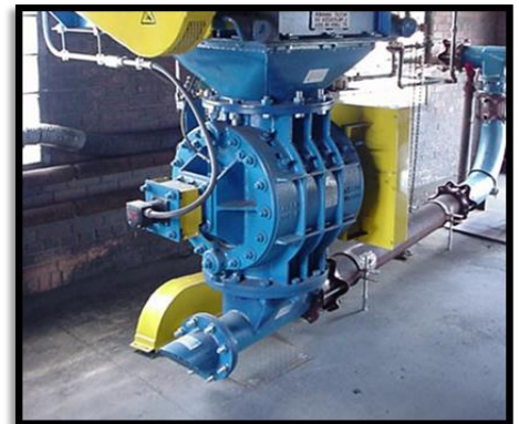
XL Rotary Valve feeding a vacuum conveying line at a pick-up point
